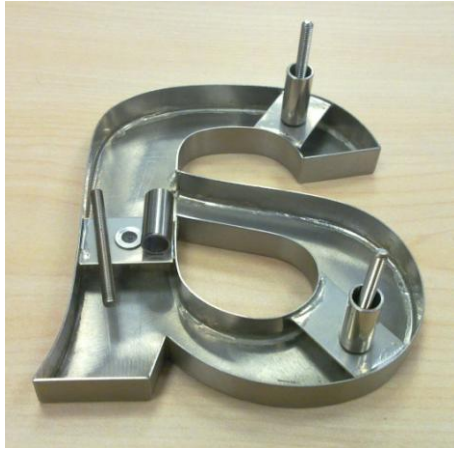
Back of letters with studs, spacers & template
